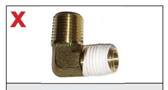
**DO NOT** use Teflon sealing tape or hand tools to install the fittings that screw directly into the pump head. The excesive stress to the threaded pump ports will lead to immediate head cracking.
